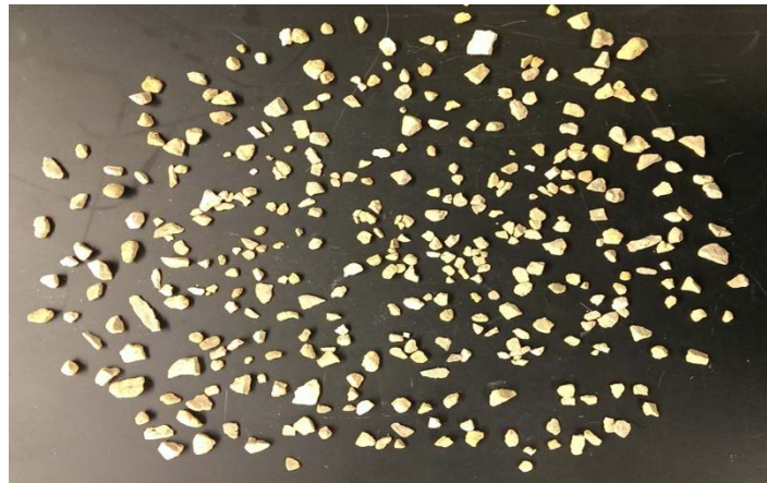
Figure. 1. Aggregate particles treated with PU
