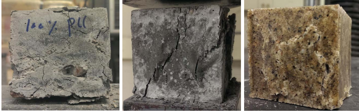
Fig.5 (a) 100% PU sample after compression test (b) Poly (vinyl alcohol co-ethylene) sample after compression test (c) Neat Resin sample after compression test
